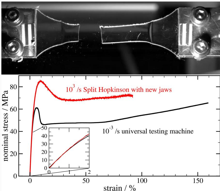
Top: Snapshot of a tensile test of a Polycarbonate specimen, torn apart at high velocity and filmed with a high-speed camera.
